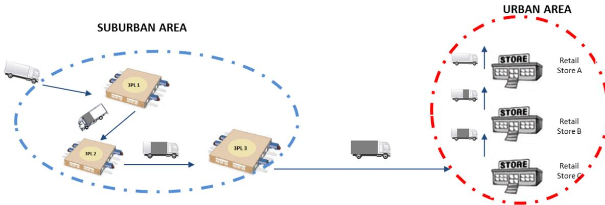
Delivery of goods into urban areas can be organized either by direct transport (Figure 2) or by using UCCs (Urban Consolidation Centre's) for consolidated transport (Figure 3). The UCC concept enables the shipper to use full-truck-load (FTL) transport for long haul to the consolidation point outside the city. Afterwards, routes are created for smaller vehicles to deliver inside the city using the “milk-run” principle.
