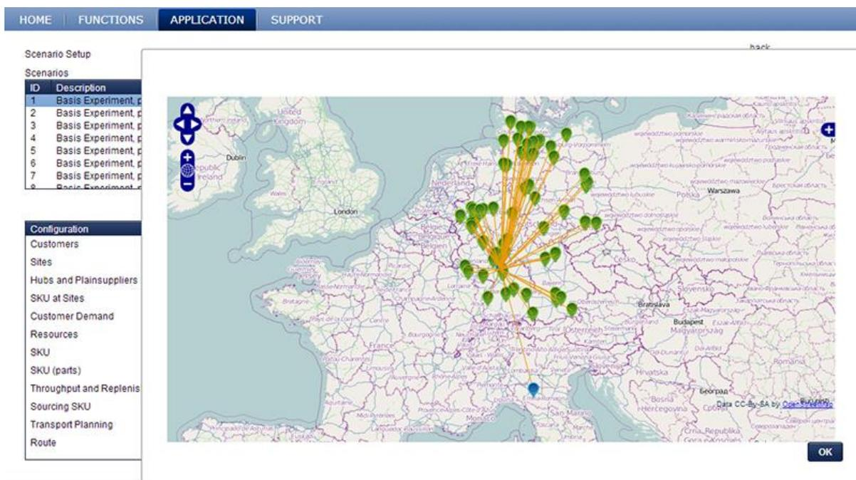
With the help of the simulation, different collaboration scenarios will be evaluated. Comparing the results from these scenarios allows us to assess which approaches deliver benefits and keep cost increases to a minimum. For the scenario comparison, different performance indicators are available: service level, transport costs, number of vehicles, number of deliveries and delivered SKUs.
